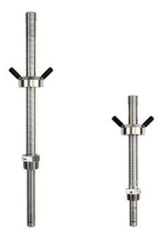
The Signet 2552 Metal Magmeter from Georg Fischer features all-stainless steel construction. The PVDF nosepiece and FPM O-rings are the only other wetted materials. The 2552 installs quickly into standard 1½ in. or 1½ in. pipe outlets, and is adjustable to fit pipes from DN50 to DN2550 (2 to 102 inches). Two sensor lengths allow maximum flexibility to accommodate a variety of hardware configurations, including ball valves for hot-tap installations.
